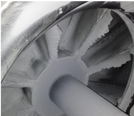
Fig.1 The original fan rotor required sandblasting every 2-3 weeks to remove hard build-up.
