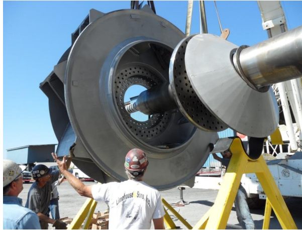
Fig. 4. The new 152.75" diameter rotor delivers a 10% volume flow increase and 16% efficiency improvement at the new high temperature operation, in the existing fan housing.
